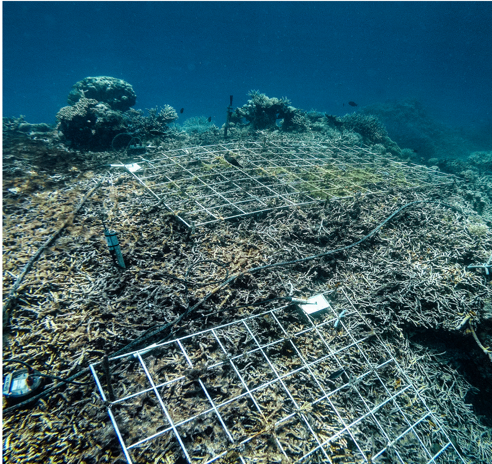
Quicksilver Group's scientifically innovative Reef Restoration Research Project aims to preserve the significant ecological, social, and economic value of the GBR World Heritage Area by transplanting corals onto low-voltage metallic mesh to facilitate the deposit of calcium carbonate and stimulate the growth of coral skeletons.
